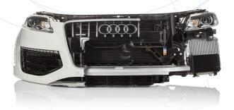
The front-end module is a complex assembly at the front of the vehicle, which, from a technical front-end, includes the shock absorption beam, the lighting and engine cooling systems, the active radiator grille shutters and the driving assistance radars and sensors.
