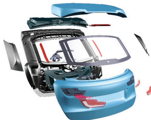
Carbon reinforced tailgate - a 10% weight reduction compared to progress already made with all-aluminium design
