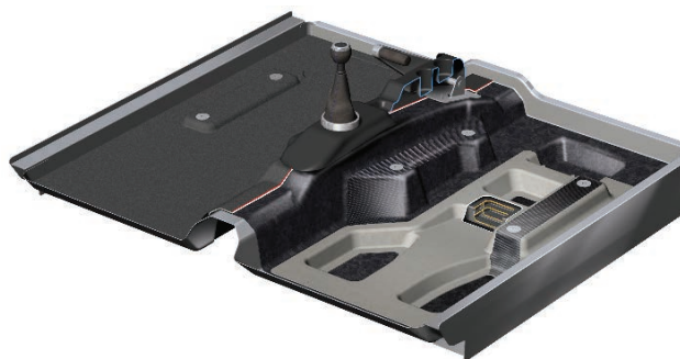
On-line high performance composite main floor
