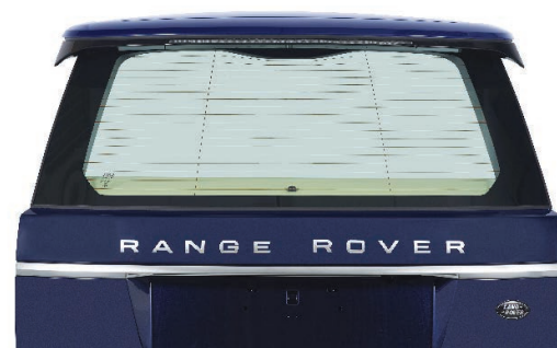
Range Rover Higate - hybrid thermoplastic/thermoset tailgate
