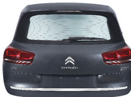
Citroën C4 Picasso Higate - hybrid tailgate molded in color
