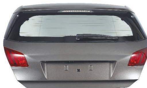
Peugeot 308 - full thermoplastic tailgate
