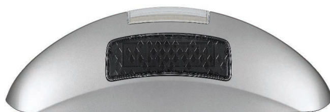
Nissan Leaf roof spoiler - large and complex painted body panel part
