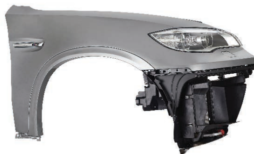
BMW X5 fender - thermoplastic injection molded
