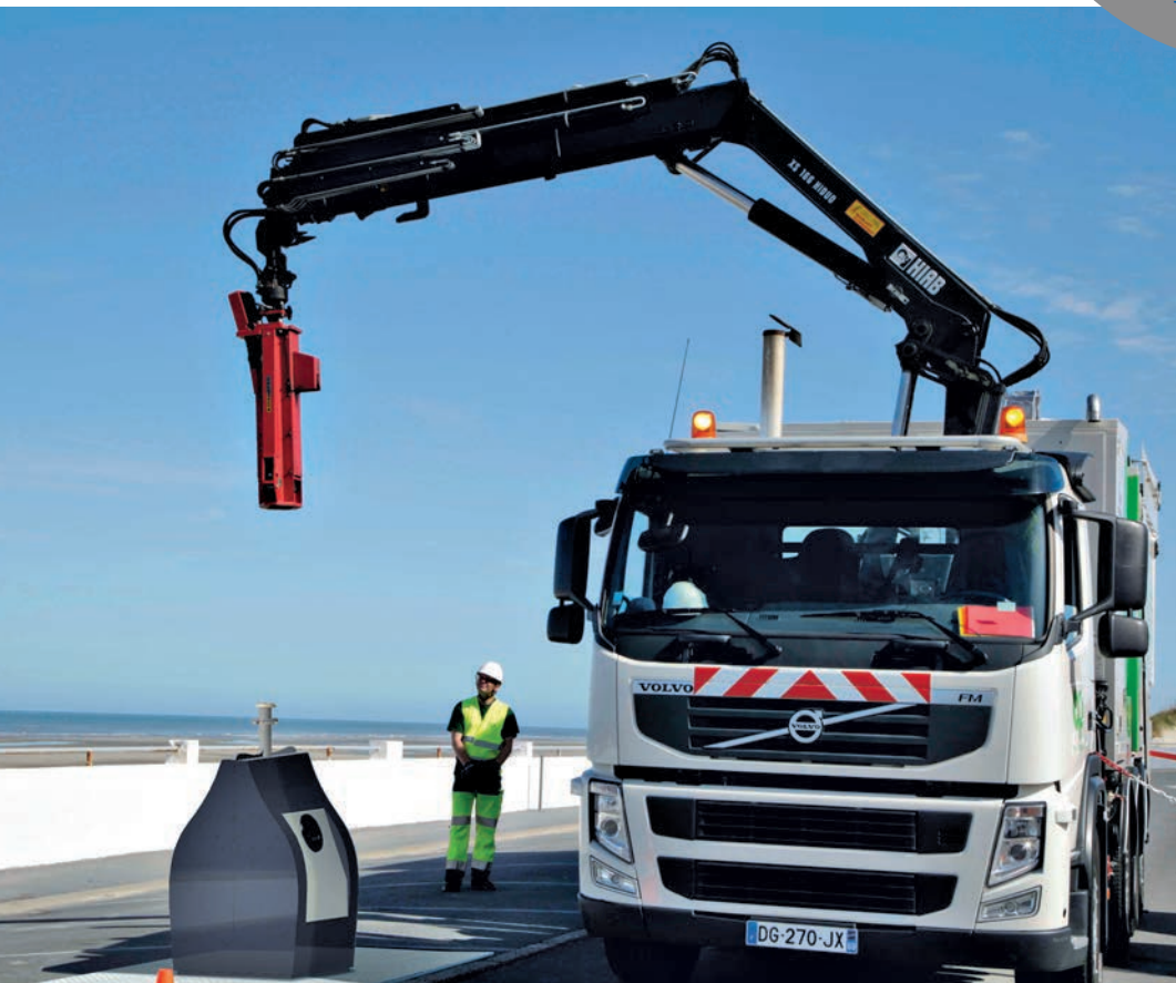
Washing trucks for underground containers provide efficient and ecological maintenance, multiplying the equipment's useful life threefold.
