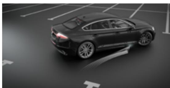
This is the first projection module in the world to use a microlens system for non-static lighting on the ground next to a vehicle.
