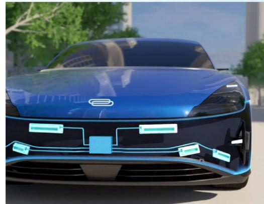
**4D imaging radar** that can interpret surroundings in 3D and real-time, no matter the weather conditions.
