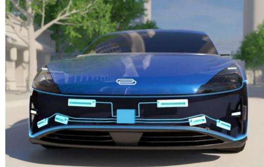
Greenerwave has developed wave control technology that paves the way to designing a new generation of automotive radar. Plastic Omnium has mastered the large-scale production of this technology, as well as its integration into plastic body parts.
