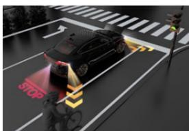
Exterior projection systems enhance traditional lighting functions in relevant situations. **Our Dynamic Turn Signal Projection**, for example, projects the turn signal onto the road next to the vehicle to improve visibility and thus provide additional safety for other road users.
