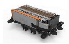
The 48V battery from OPmobility is a battery for mild hybrid cars and hybrid electric trucks. This power battery uses NMC lithiumion cells and recharges itself, mainly when decelerating and braking. Electrical energy is used to assist the internal combustion engine, particularly when accelerating, helping to cut tailpipe C0<sub>2</sub> emissions by up to 15%.
